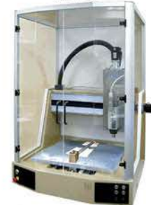
Specimen milling Machine for machining of plastic test specimens for tensile and impact tests
